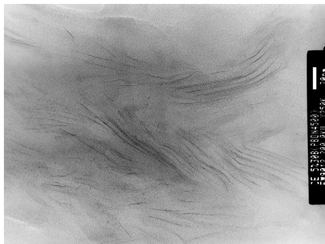
Fig. 11. TEM picture related to a quasi-exfoliated nanocomposite based on CE and Cloisite 30B modified with LPB-3-M7.5.
