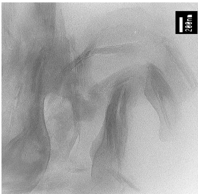
Fig. 9. TEM picture related to an intercalated nanocomposite based on CE and Cloisite 30B.
