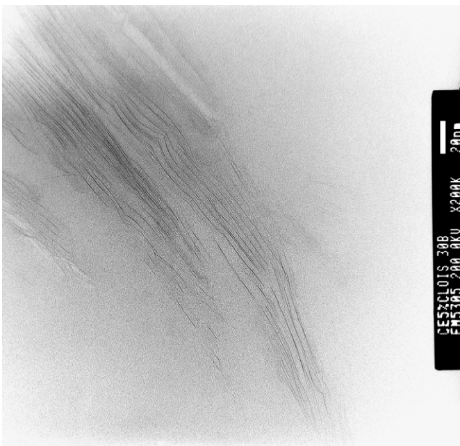
Fig. 10. TEM picture related to an intercalated tactoid of Cloisite 30B in UV-cured CE.
